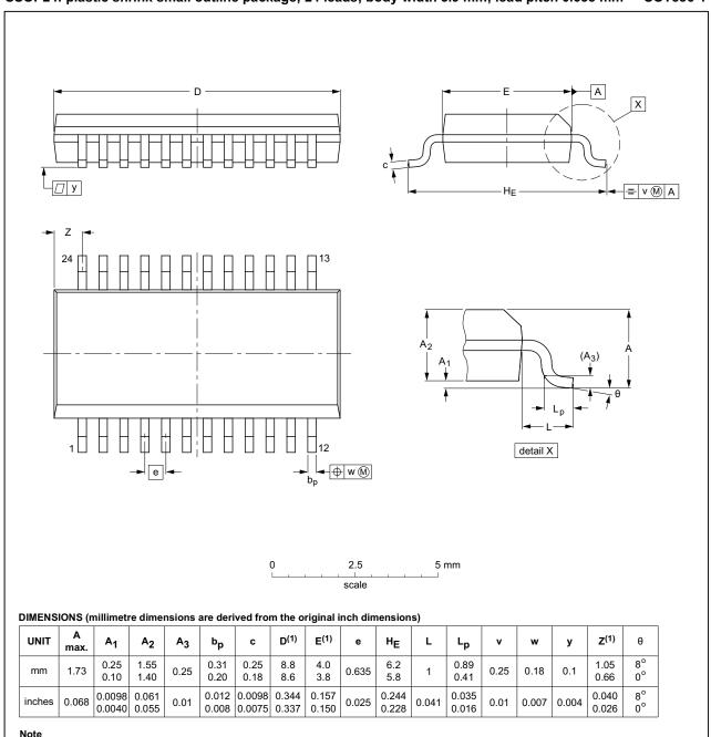
1. Plastic or metal protrusions of 0.2 mm (0.008 inch) maximum per side are not included.
