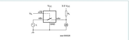
nOE connected to GND; Adjust f<sub>i</sub> voltage to obtain 0 dBm level at output. Increase f<sub>i</sub> frequency until dB meter reads –3 dB.
