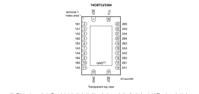
(1) This is not a supply pin. The substrate is attached to this pad using conductive die attach material. There is no electrical or mechanical requirement to solder this pad. However, if it is soldered, the solder land should remain floating or be connected to GND.
