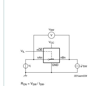
Fig 8. Test circuit for measuring ON resistance (one switch)
